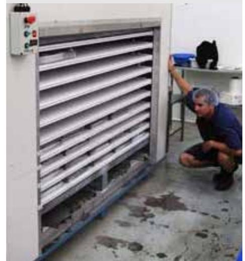
Custom built plate evaporators are used to snap freeze the produce.
